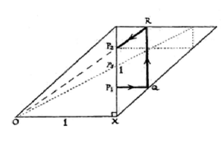
Draw a parallelogram as shown. Take any point P1 on the vertical line. Draw P<sub>1</sub>Q horizontally and QR vertically. Draw from R towards O to find a new point on the vertical line, P2. Repeat the process taking P<sub>2</sub> as your new starting point.
