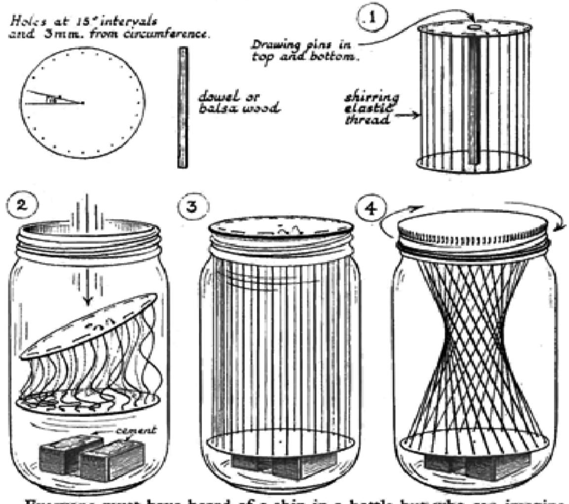
Everyone must have heard of a ship in a bottle but who can imagine a mathematical model in a jar? The main requirements for this model are a cylindrical jar, some stiff card, shirring elastic thread and a piece of dowel.
