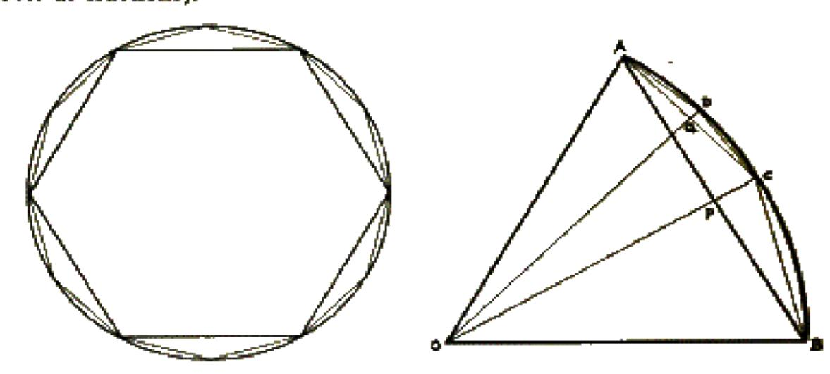
We can start by fitting a regular hexagon inside a circle of unit radius. In the figure ABO is an equilateral triangle and P is the mid-point of AB. Therefore AP is 0.5 inches.
